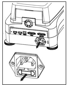
Using a test pen, turn the fuse holder to the left (counterclockwise) and remove the fuse.
