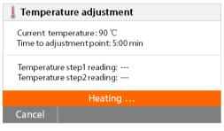
The dryer unit is heated to a temperature of 100°C. You can observe the progress on the display as the dryer temperature and count down period are displayed. After 15 minutes, read the thermometer through the inspection window on the cover and enter this temperature. Adjust the display reading to agree with the thermometer, then press the **Enter** button. You have 15 minutes to make this adjustment, otherwise the adjustment is terminated.
